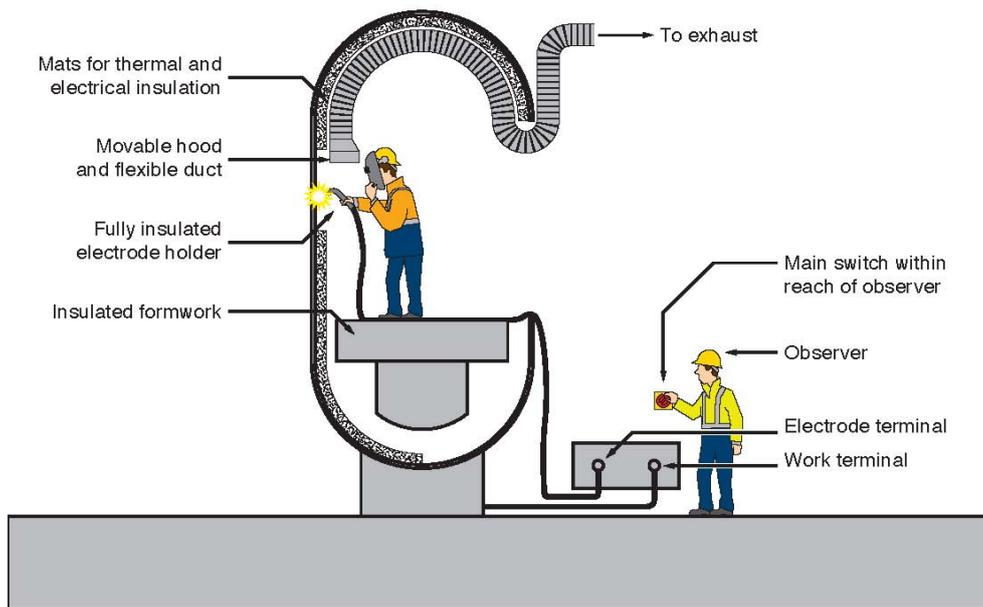
**Figure 1: Local Exhaust ventilation in confined space welding**
