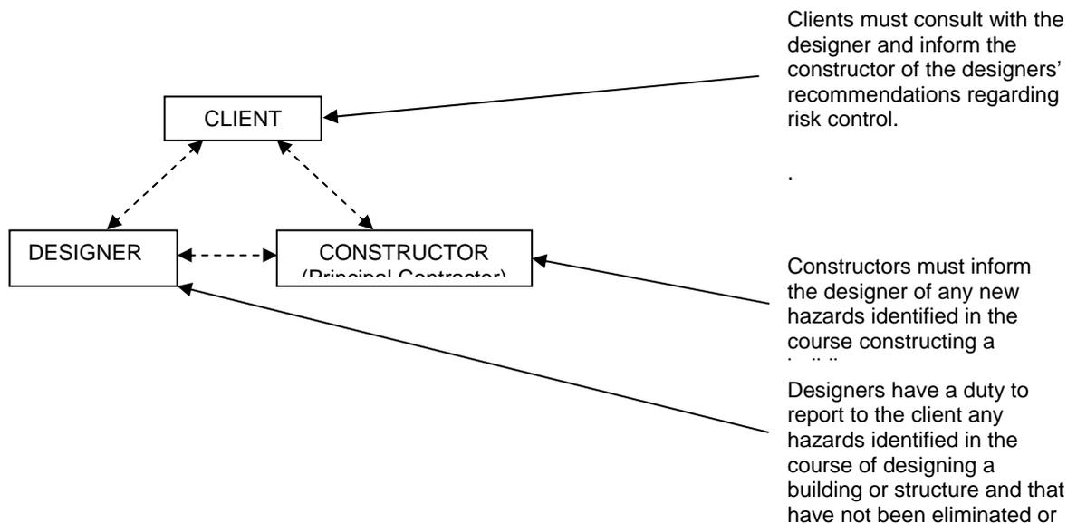
**Figure 2d – This model may apply to a complex construction project such as a hospital or airport terminal where specialist contractors carry out large parts of the project**
