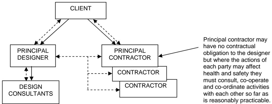
**Figure 2e – This model may apply to large construction projects where the management role is carried out by a specialist construction manager**
